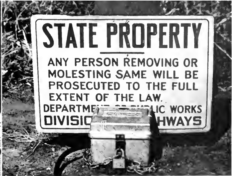
Top photo shows typical installation of automatic traffic counter on highway. Black line on pavement in foreground is 9/16 inch rubber tubing that actuates counting machine. Lower pictures show recording mechanism in box which is secured to post by lock and chain
